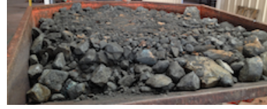
Fig. 6. Photo of the soil material used in the experiments inside the metallic container. Different sizes of rock can be seen making up the propagation domain \Omega_2 .
